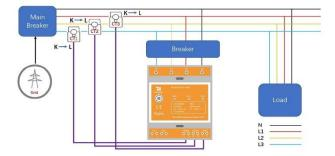
In the above wiring diagram the three CT clamps are clamped around Phase A, B, C of the main incoming three phase line from Eskom (the grid). But you could also move them to L1, L2 and L3 of a specific load to measure just that device or circuit.
