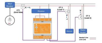
In the above wiring diagram the device is clamped around the main incoming line from Eskom (the grid), as well as Load1 and Load2.
